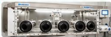
Glove Box (Argon Atmosphere) (2 persons can work simultaneously)
